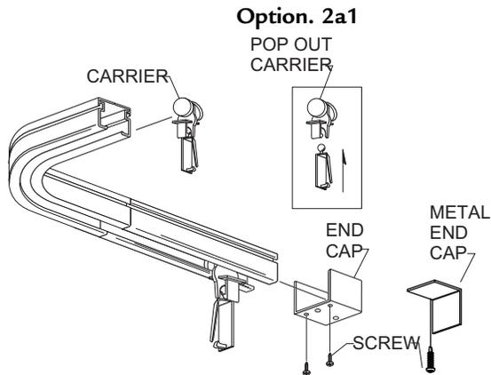
2. Slide the carriers on the track and attach end caps (plastic or metal) on the open ends. SEE FIG. 5
